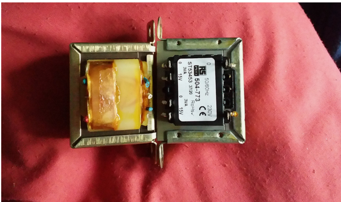
Figure three, above: Old transformer (left) and replacement from RS Components (right).
